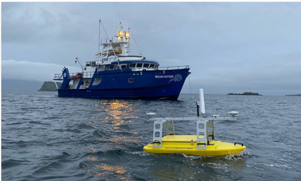
The EchoBoat-160 (affectionately dubbed the R/V Sea Lemon) is a bright yellow Autonomous Surface Vehicle (ASV) equipped with a multibeam sonar, complete with programmable survey paths and capable of mapping shallow or rocky waters that would otherwise be challenging for boats to navigate. NPS Coastal ecologists in the Alaska Region are using the ASV for offshore mapping that overlaps with long-term monitoring sites to provide a continuous dataset from exposed land on shore to submerged land, including seagrass, sand flats, and rocky habitats. One use of the data will be to determine factors connecting sea otter density and preferred habitat selection. Monique LaFrance Bartley, NPS. Learn more: https://www.nps.gov/im/sean/monitoring.htm
