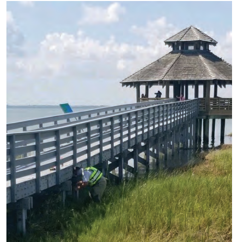
USGS Hydrologic Technician Mark Warzecha, installs a storm surge sensor in Port Lavaca, TX, in advance of Hurricane Marco’s landfall along the Gulf of Mexico’s northern coast. Photo credit: Alex Laffoon, USGS
