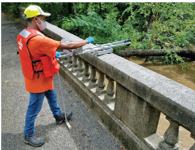
USGS hydrologic technicians Fisseha Mengistu (at left), lowers a water sampler into Rock Creek in Washington, D.C., to collect samples to track how Isaias affected water quality and Logan Jeffries (at right) uses a hand-held instrument called an Acoustic Doppler Velocimeter to measure streamflow August 4 on Tenmile Creek near Clarksburg, MD. Photo credits: Erica Warner, USGS (left), Matt Baker, USGS (right)
