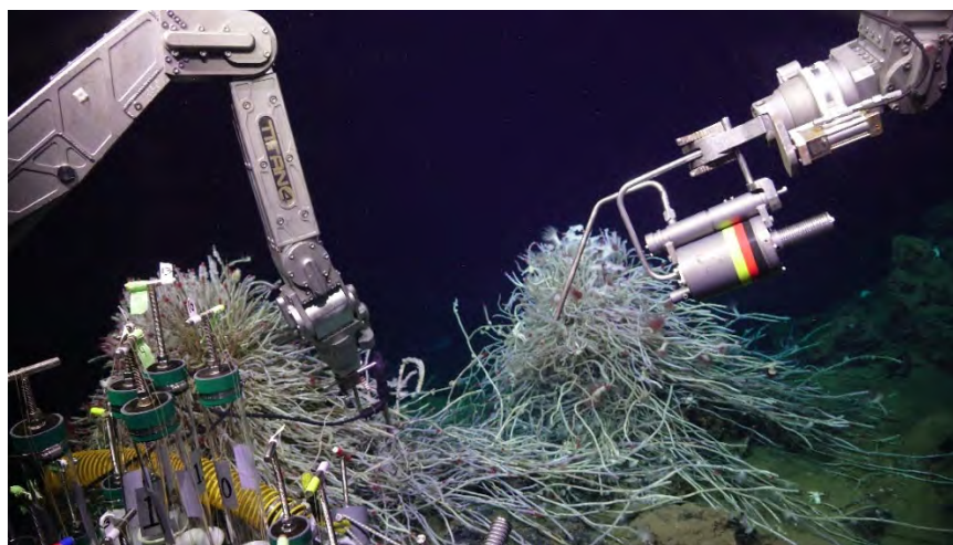
The Jason ROV sampling a hydrothermal vent situated inside a cluster of tubeworms at a depth of approximately 3200 meters.
