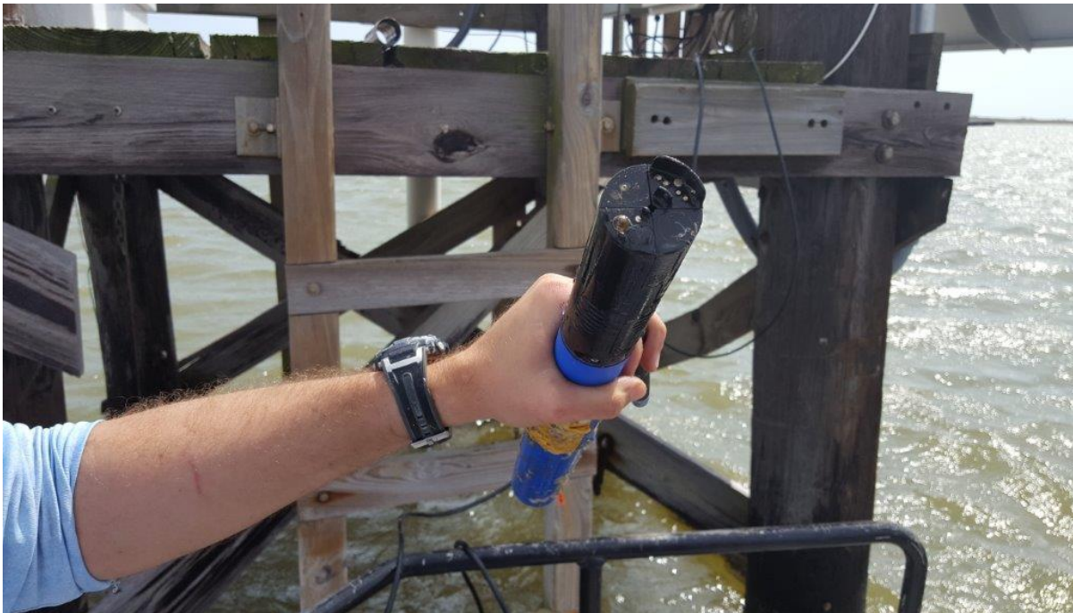
Since 2010, the Gulf Coast Inventory and Monitoring Network has continuously monitored water quality in an extremely high biofouling environment at Padre Island National Seashore. Upon replacing the standard instruments with two NPS-modified instruments, the Network reduced maintenance costs by over 50 percent. These images show the results of a 6-month proof-of-concept deployment: above left, biofouling on the outside of the instrument; above right, the instrument after scraping material off the outside; and above center, the sensors on the inside of the instrument with no other cleaning or maintenance. Photo: Conrad Blucher Institute, NPS partner.
