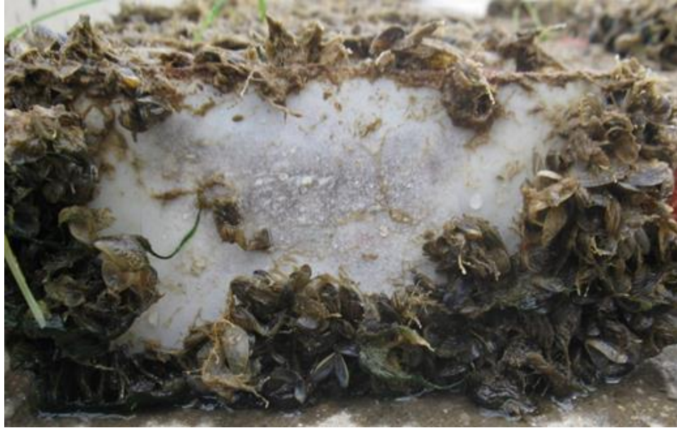
NDSU sample C4-20 installed May 2012, Photo taken July 2019. Mussels do not adhere to the coating surface but can attach to the algae that is on the coated surface. Mussels are firmly attached to surrounding, non-coating surfaces. Photo: Bureau of Reclamation.
