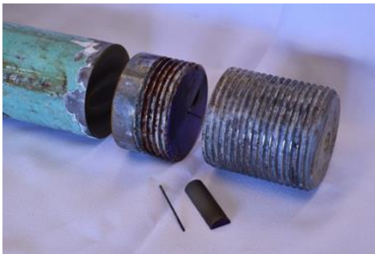
Subsea stud cut for X-Ray Characterization. Credit: BSEE/Argonne National Laboratory (ANL) Research
