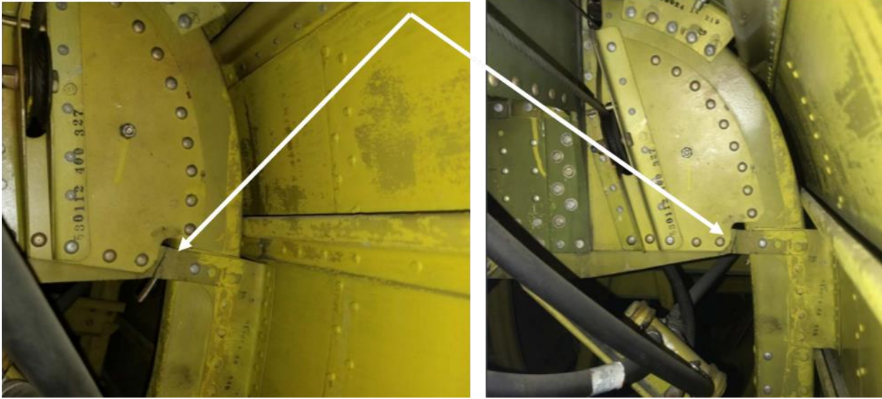
Figure 4. Cracks in aircraft bulkhead.
