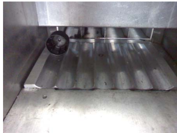
Figures 2 and 3. Cap blocking the #1 chute.
