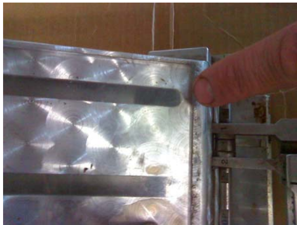
Figures 2 and 3. Cap blocking the #1 chute.
